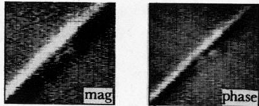
FIGURE 2. Thermal wave transmission image (magnitude and phase) of a seam in 0.1 mm stainless steel.
