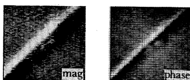
FIGURE 2. Thermal wave transmission image (magnitude and phase) of a seam in 0.1 mm stainless steel.
